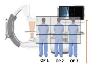
The image shows the locations of each operator. Operator position 1 is 28 inches down the table from the x-ray tube. Operator position 2 is 56 inches, and operator position 3 is 80 inches. When the Rampart M1128 V2.0 is placed, it is 10 inches down the table from the x-ray tube.
