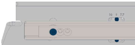
Accessory Rail Set to 9.0 mm Size
